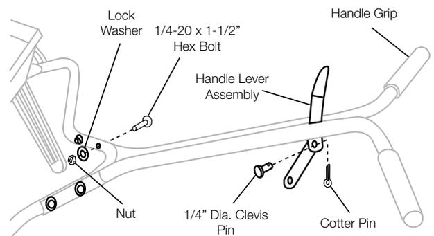
**5.** Slide the ends of the Control Tube Braces over the studs on the Shutoff Bar Brackets, secure with Cotter Pins. Attached opposite end of Control Tube to the Handle Lever using 1/4 dia. Clevis and Cotter Pin. Make sure Handle Lever operates freely. **Tighten all Nuts left loose in Step 1.**
