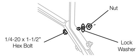
**4.** Stand spreader upright on Wheels. Attach Upper Handle assembly to Handle Brace (make sure Handle is positioned as shown) using (4) 1/4-20 x 1-1/2" Hex Bolts, (4) Lock Washers, and (4) Nuts. Tighten securely. Install Handle Grips onto Upper Handle. Slide Handle Lever assembly between Handle Brackets and secure with 1/4 dia. Clevis and Cotter Pin. Make sure Lever pivots freely.
