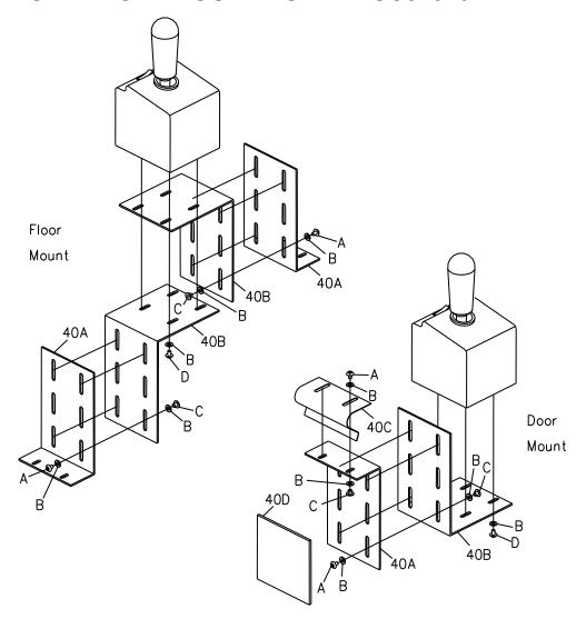
Figure 39. Joystick Control Universal Mounting Kit Components
