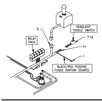
Figure 20. Internal Cab Wires
