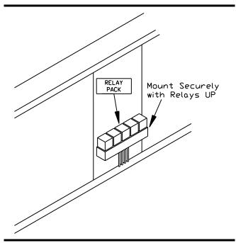
Figure 24. Relay Mounting.
