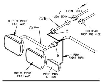
Figure 28. Dual Headlight Adapter Connections
