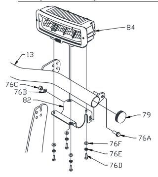
Figure 11. Headlight Mounting Assembly
