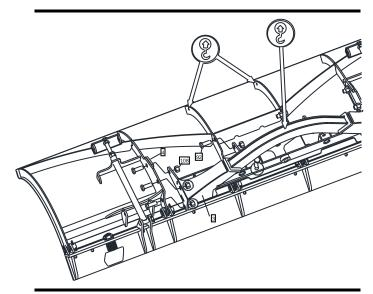
Figure 3. Install Pushframe Attachment Bar
