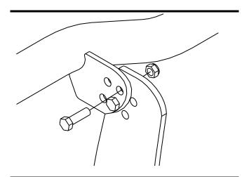
Figure 10. Light Bar Assembly Adjustment.
