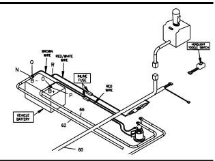
Figure 22. Battery Connections
