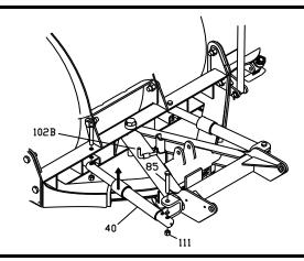
Figure 5. Install Angle Cylinders
