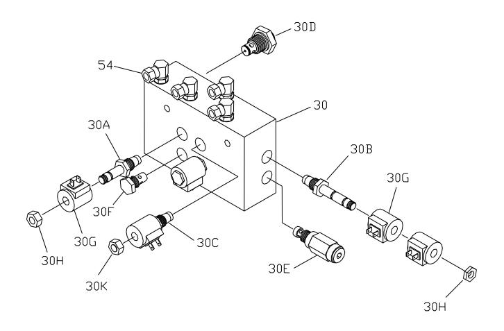
Figure 37. Straight Blade Manifold with SmartHitch2™ Parts Diagram
