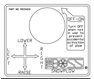
Figure 38. Straight Blade Control Operation
