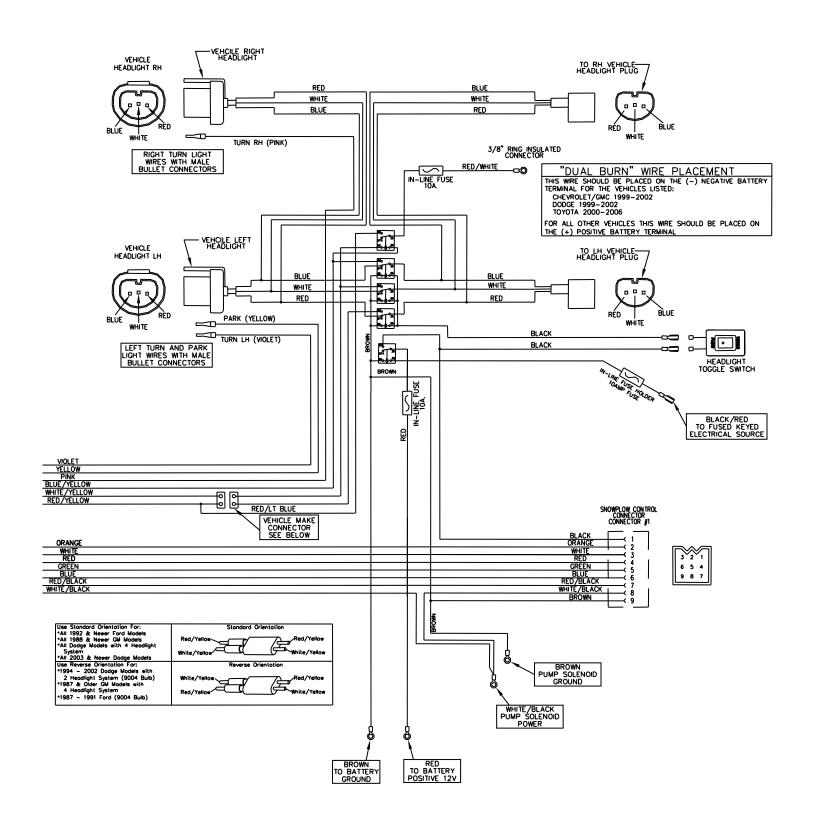
Figure 30. Electrical System Wiring Schematic (Truck Side)
