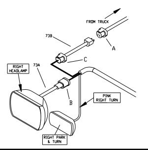
Figure 27. Single Headlight Adapter Connections G10149
