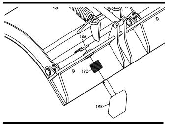
Figure 2. Install Shoe Assembly
