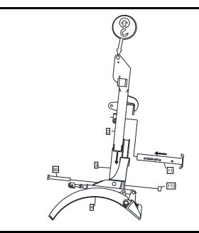
Figure 4. Install Pushframe and Kickstand.
