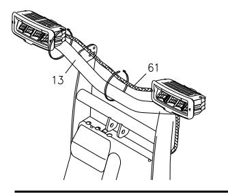
Figure 12. Securing Wiring Harness
