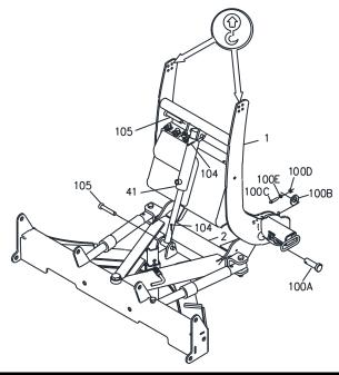
Figure 6. Lift Cylinder Installation
