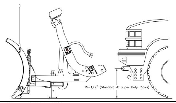
Figure 42. Recommended Pushbeam Height
