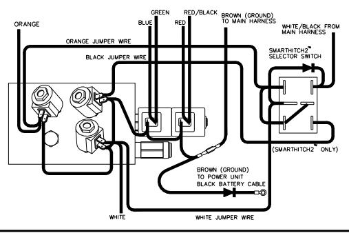
Figure 33. HYD07091 Super Duty Manifold Wiring Diagram
