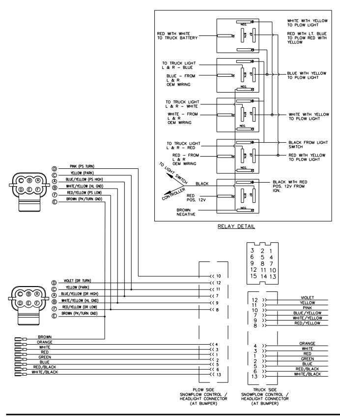
Figure 29. Electrical System Wiring Schematic (Plow Side)
