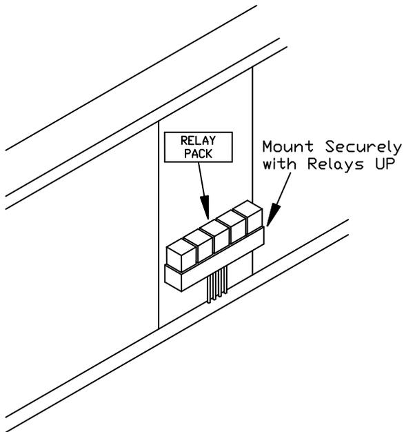
**Figure 21.** Relay Mounting. G10052
