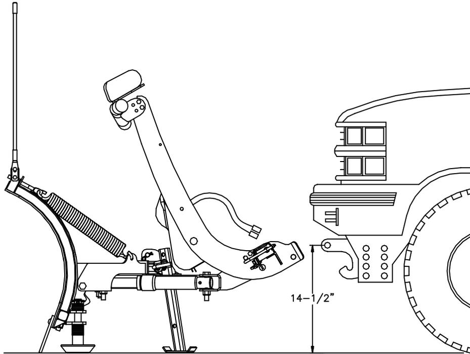
Figure 39. Recommended Push Beam Height- Sport Duty
