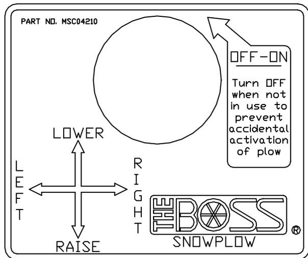
**Figure 35.** Straight Blade Control Operation G10154
