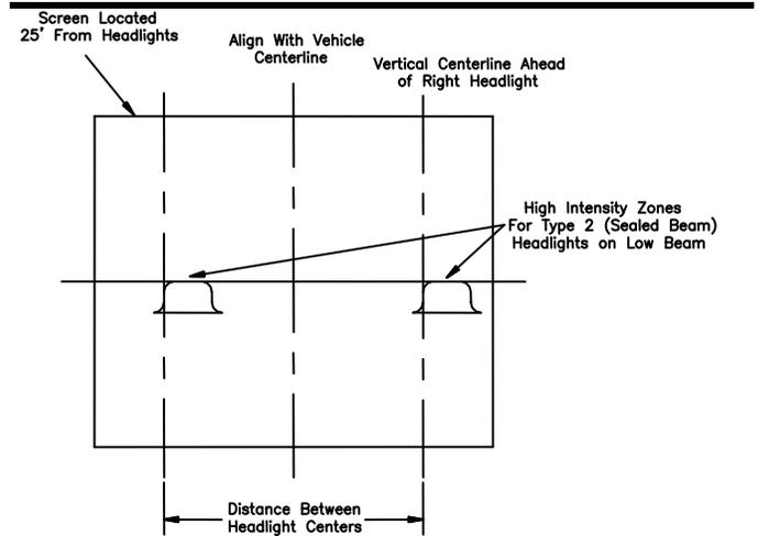
Figure 33. Headlight Aiming Procedure
