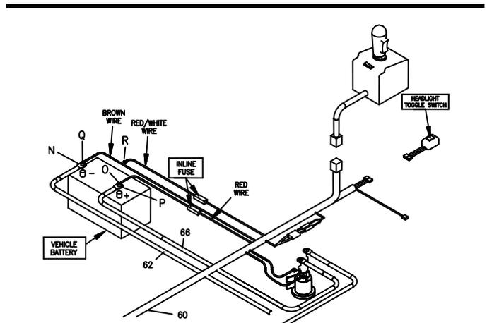
**Figure 19.** Battery Connections G10146
