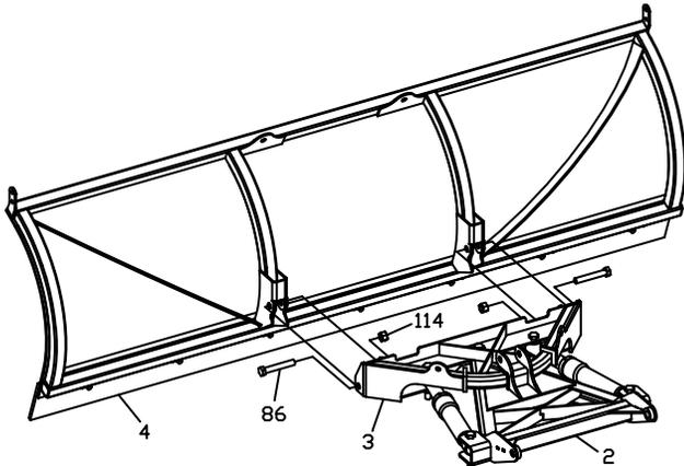
**Figure 2.** Push Frame Attachment G10298
