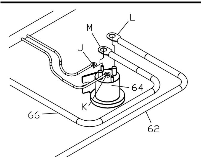
**Figure 18.** Solenoid Connections. G10145
