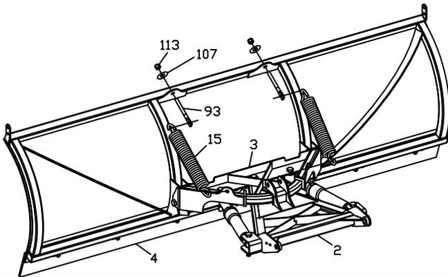
**Figure 3.** Trip Spring Assembly G10300
