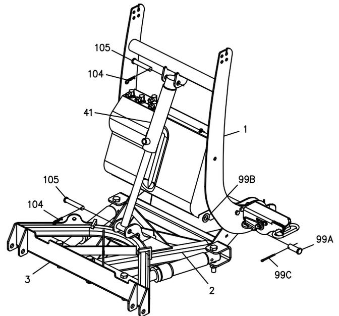
**Figure 4.** Lift Cylinder Installation G10301
