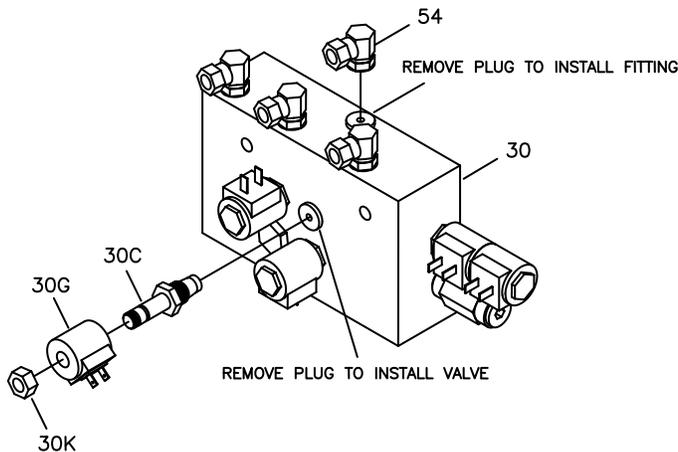
**Figure 11.** SmartHitch2™ Valve Installation G10130
