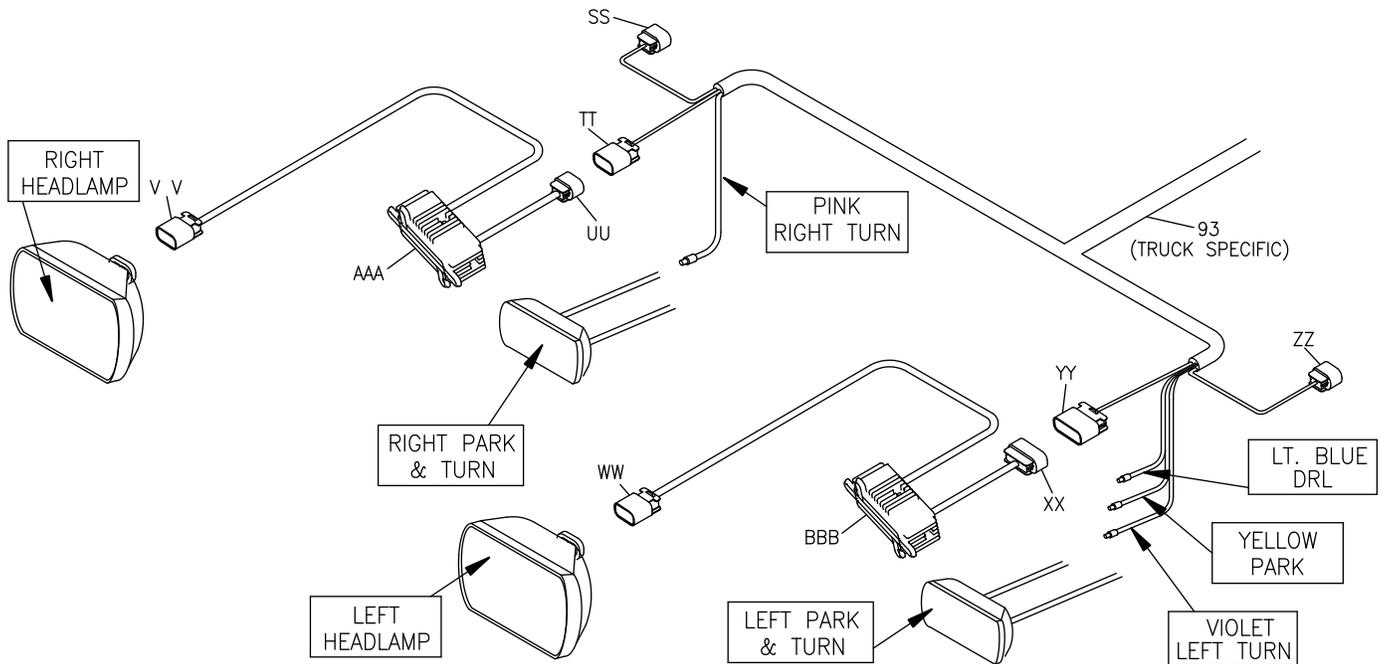
Figure 9: Headlight Resistor Wiring
