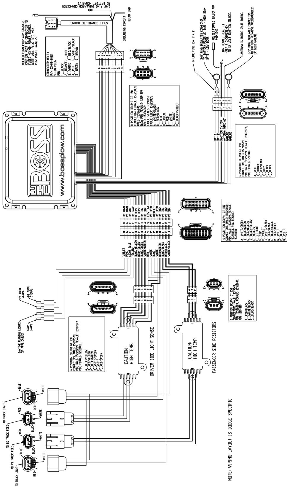
Figure 17: Electrical System Wiring Schematic (Truck Side with Resistor Boxes)
