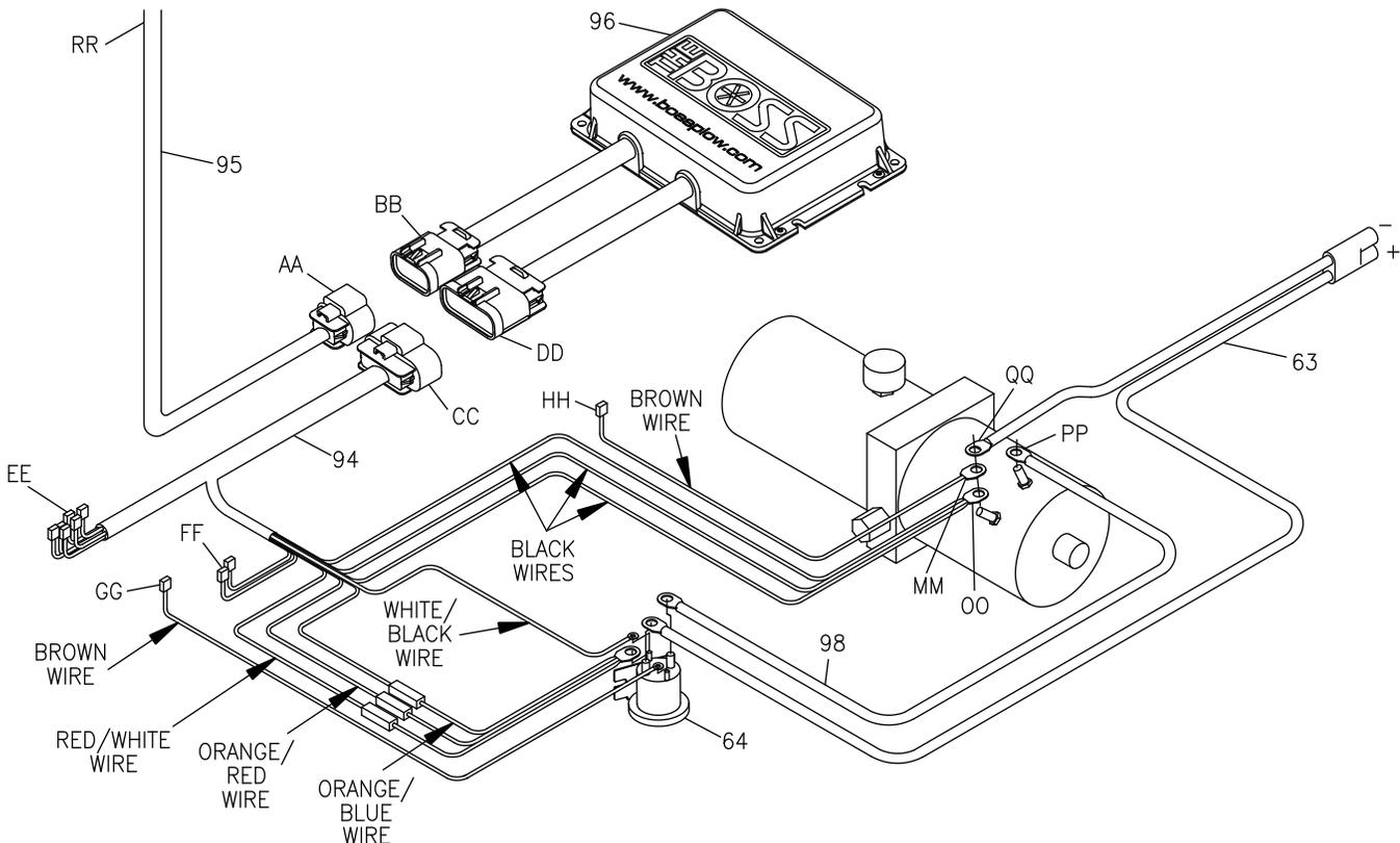
Figure 10: Plow Side Wiring
