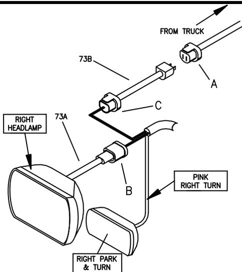
Figure 7: Single Headlight Adapter Connections G10149
