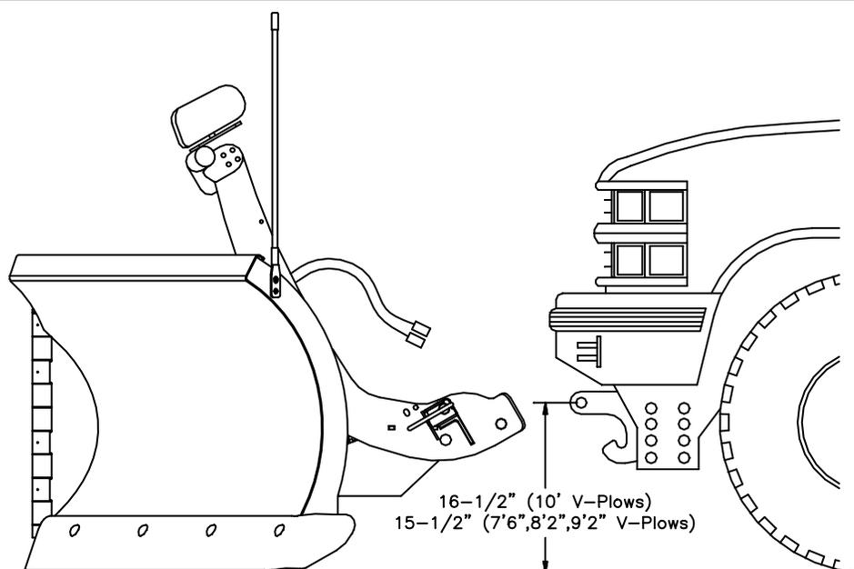
Figure 24. Recommended Push Beam Height
