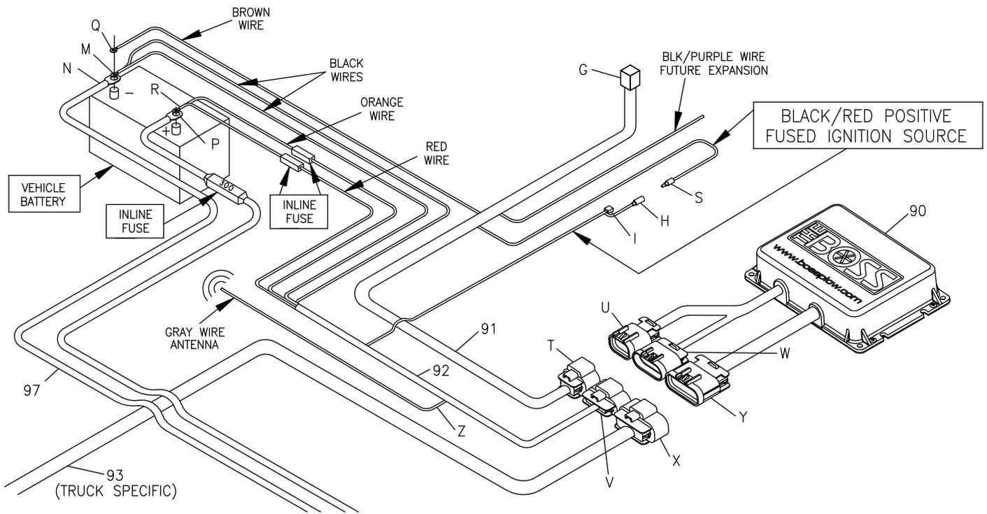
**Figure 5:** Internal Cab Wires
