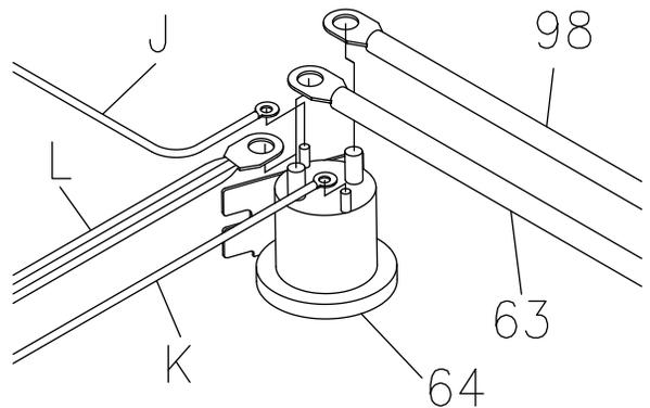
**Figure 13:** Solenoid Wiring
