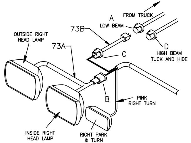
Figure 8: Dual Headlight Adapter Connections G10151
