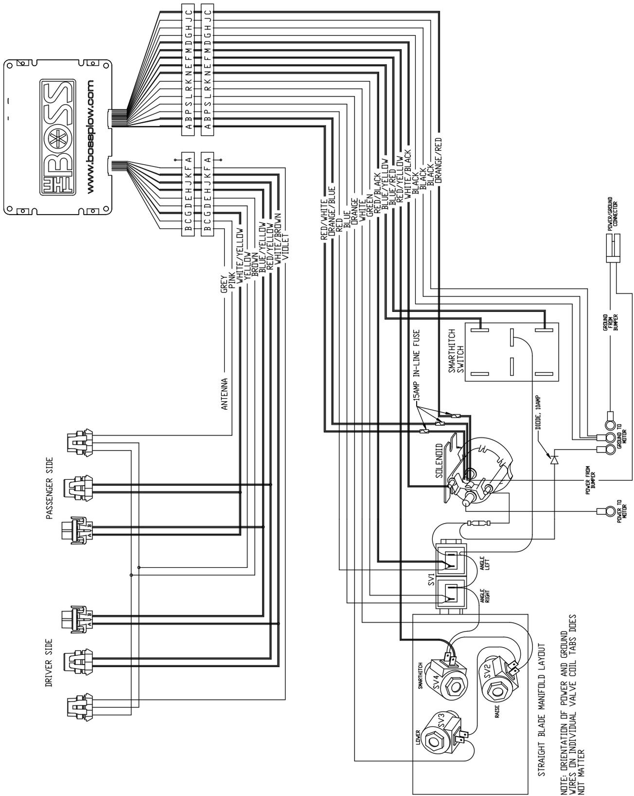
Figure 14: Electrical System Wiring Schematic (Plow Side Straight Blade)
