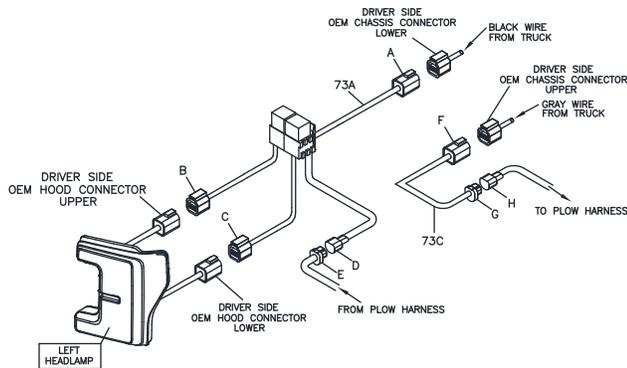
**Figure 1.** Ford Super-Duty LED Headlight Adapter Installation G13960
