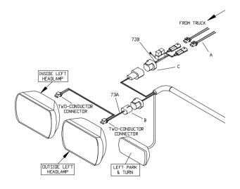
Figure 1. 1999-2002 GM Headlight Adapter Connection G10161
