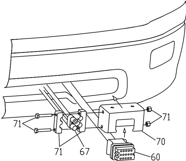
**Figure 22.** Vehicle Connections G10148
