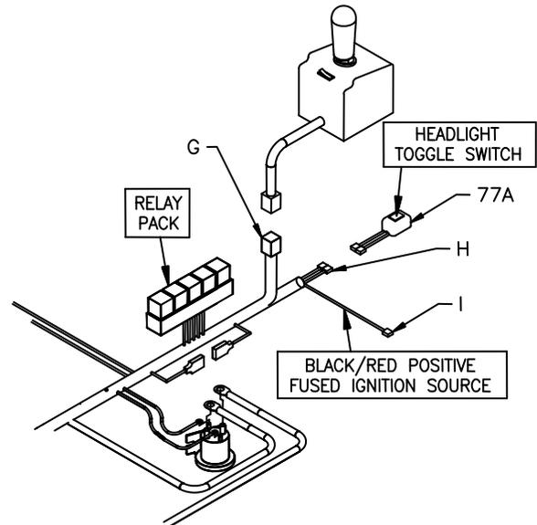
Figure 19. Internal Cab Wires
