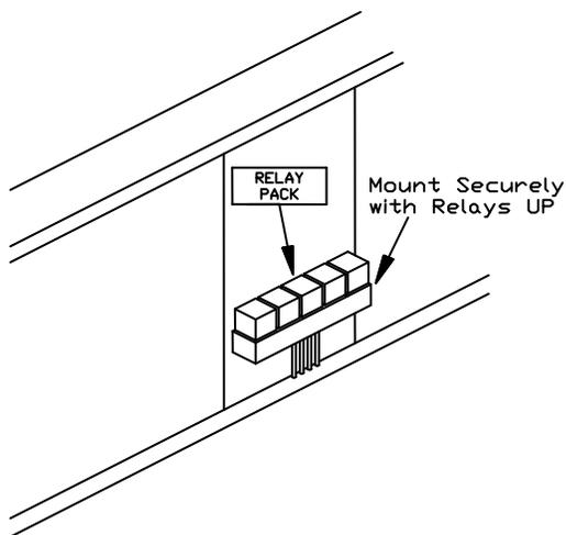
**Figure 23.** Relay Mounting. G10152
