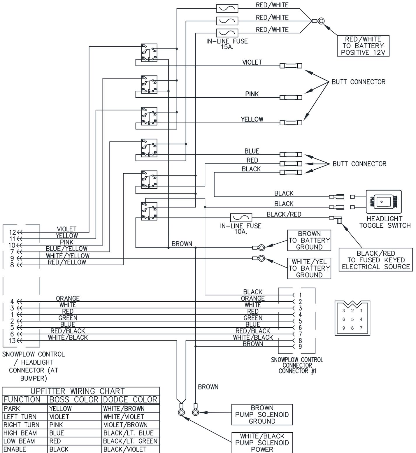
Figure 28. Electrical System Wiring Schematic (Truck Side)
