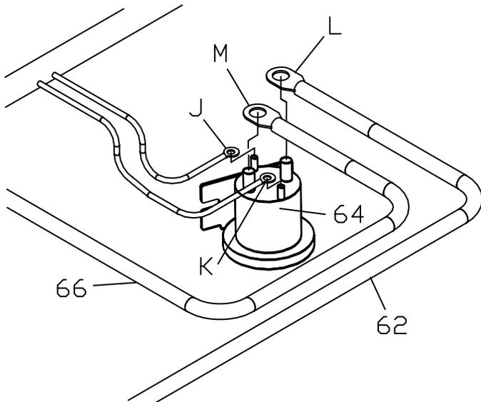
Figure 20. Solenoid Connections.
