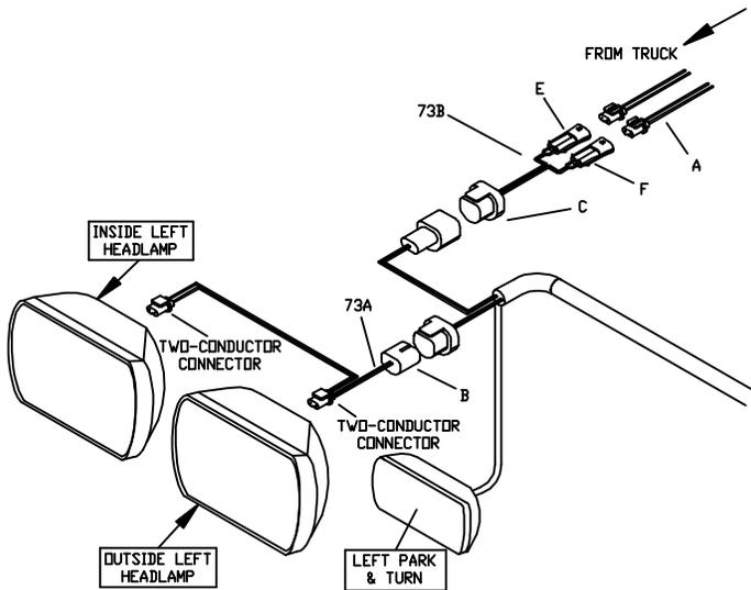
**Figure 1.** '04 & Newer Titan Headlight Adapter Connections G10161
