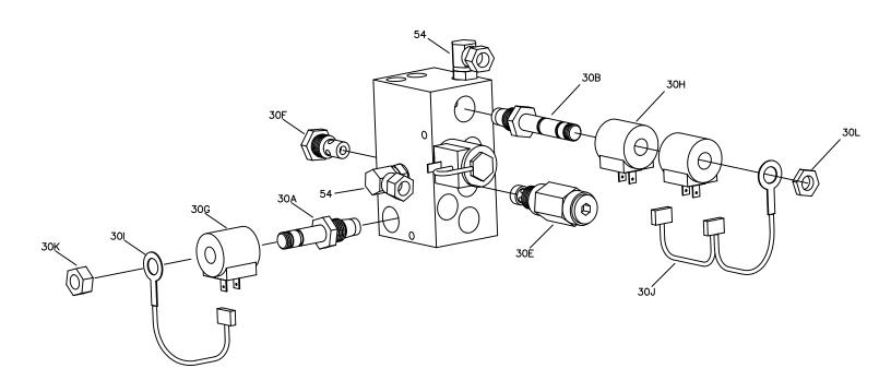
Figure 1. Hydraulic Valve Assembly Parts Breakdown
