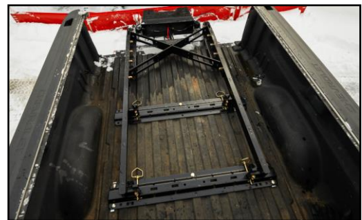
Removal of OEM tailgate and installation of aftermarket fifth-wheel Rail System is required. Rail system is not offered by BOSS
