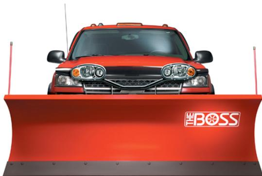
When the snow is falling and time means money, THE BOSS SmartHitch 2 is the fastest, simplest, easiest-to-use attachment system on the market. Attaching THE BOSS SmartHitch 2 is as easy as setting the lockpin levers to the “on” position, connecting the two electrical plugs and raising the light tower with a touch of a button. In addition, every BOSS Snowplow comes with a two-year warranty covering both parts and labor.
